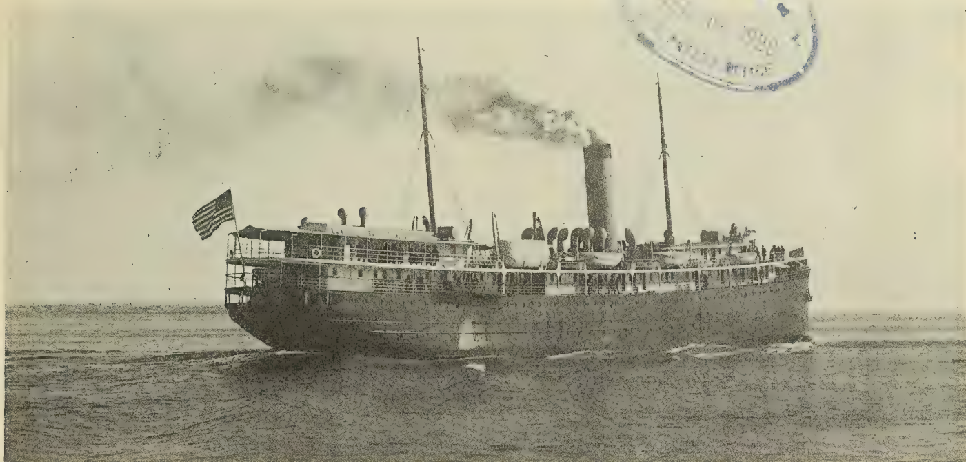
(Photograph copyright 1920 by Edwin Levick, N. Y.) Fig. 1.—S.S. Cuba, at Full Speed, Showing Flat Wake and Small Wave Formation
